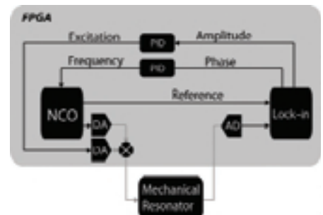
The block diagram of the PLL implemented on the FPGA illustrates the Numerical Controlled Oscillator that generates the reference and the excitation signal for the high-Q mechanical resonator. A lock-in detects phase and amplitude of the resonator's response signal. Two PID controllers track the resonance frequency and maintain the oscillation at a constant amplitude.
