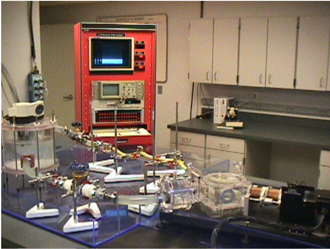
Figure 1: The LabVIEW-driven Cardiovascular Pulse Duplicator (CPD) system.
